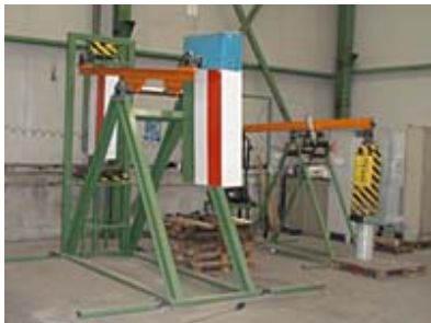
Picture 10. 1340kg Pendulum - Fondtla, Italy http://www.youtube.com/user/lla67ful
