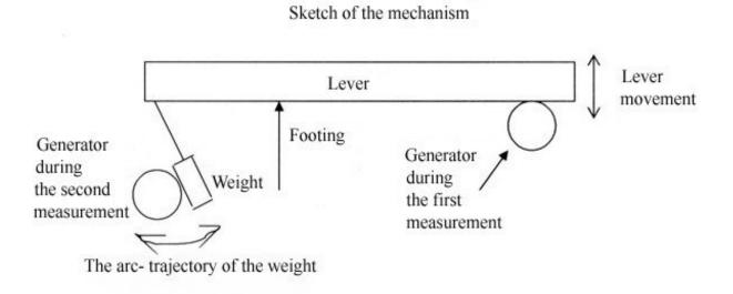
First measurement: the lever is moving the generator
